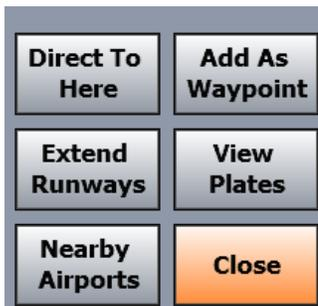
6. If needed, you can modify the flight plan by bending or **"Rubber-banding"** the route line. Touch the line at any point and drag it to a new position. You will be presented with the option to Fly Direct To or Add a Waypoint.
