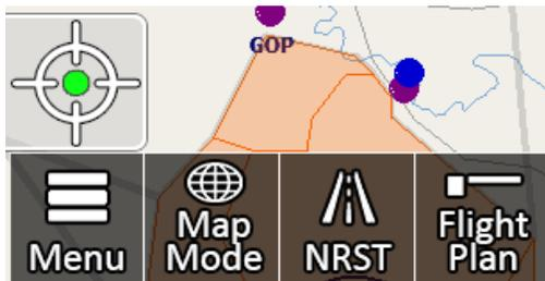
2. If there is not an active flight plan in the system, this is where you can begin to build your flight plan. Touch Enter Flight Plan and begin searching
