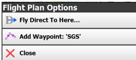
4. **Fly Direct To Here** will replace your current plan. **Add Waypoint** will add the location to the end of your plan. **Insert Waypoint** will insert into the nearest leg.
