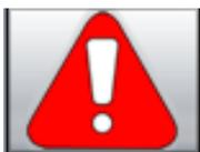
Touch the "!" button on the NRST page to enable Emergency Assist. Airports will be recommended and color-coded in Green, Yellow or Red based on the Glide Ratio entered into the Aircraft Profile.
